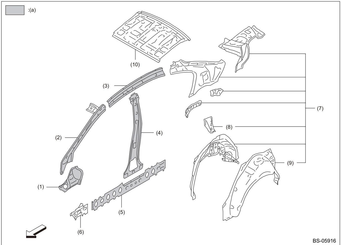
(a) High-strength tensile steel
