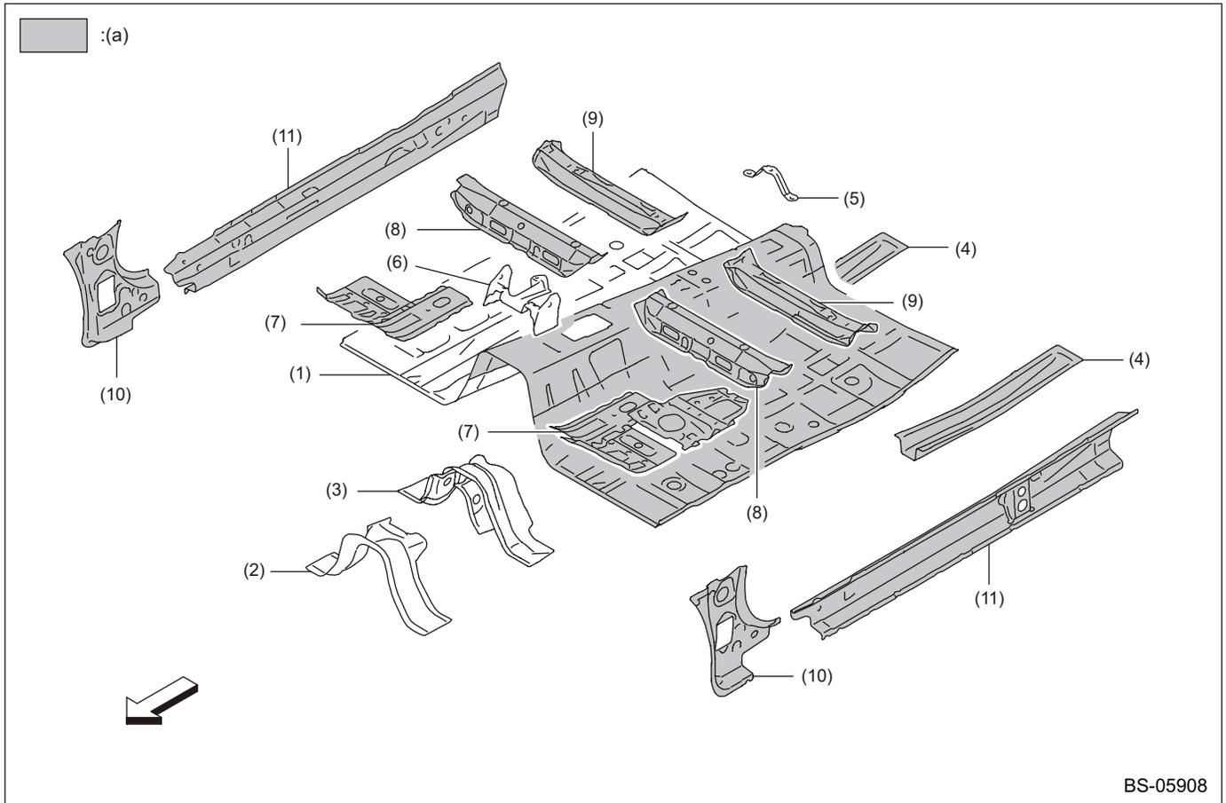
(a) High-strength tensile steel
