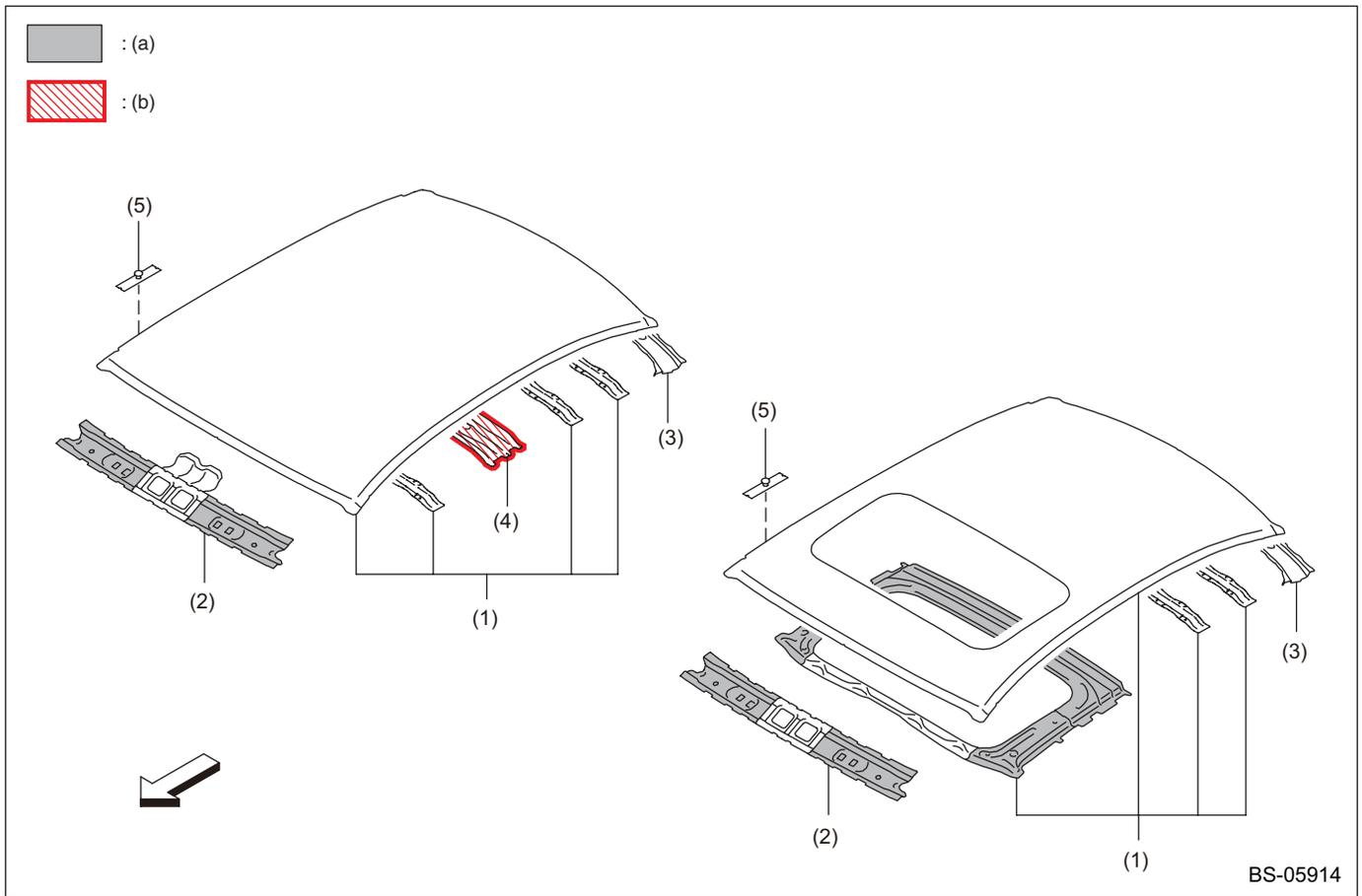
(a) High-strength tensile steel
