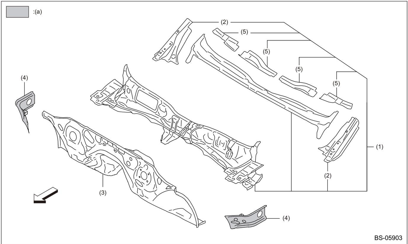
(a) High-strength tensile steel
